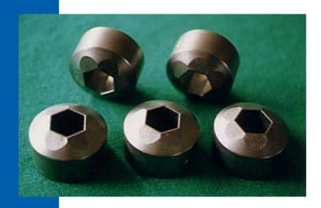
T & G Machine Tool Co., Ltd. has developed Special CVD coating (CN05) trimming dies for the longest possible life.
